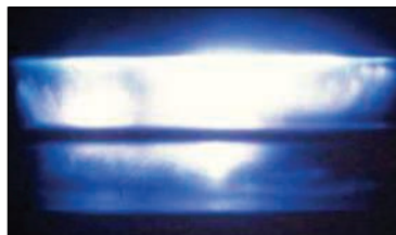
Reproduction of a historical experiment from the 18th century. The light phenomena produced through mechanical friction in a vacuum tube were considered a model of the Aurora Borealis.
